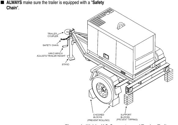
Figure 4. Welder/AC Generator and Towing Trailer
